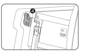
• As shown in the figure, insert the lock buckle **5** into each side, installation finished.
